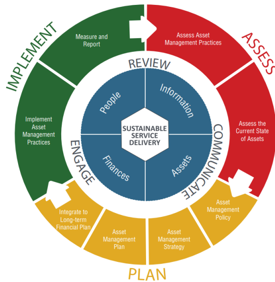
Figure 2 Asset Management Planning Process
