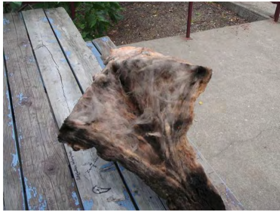
Photo 1, 2: A piece of fibrous batt insulation on the deck removed to show that the normal air pockets [provides insulation resistance] of the batt have been filled with dirt.
