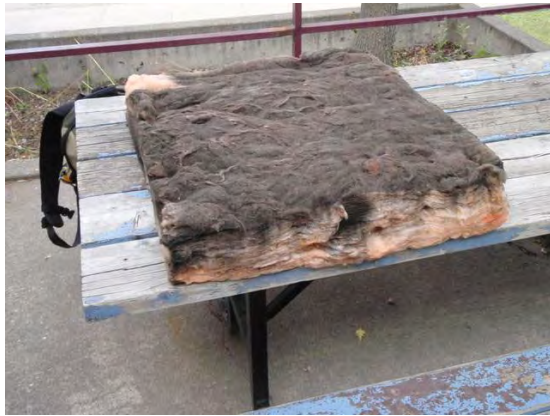
Photo 1, 2: A piece of fibrous batt insulation on the deck removed to show that the normal air pockets [provides insulation resistance] of the batt have been filled with dirt.
